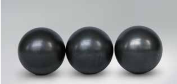
Photo 6.15.4 Part: Balls of a groove ball bearing Symptom: Electrical corrosion has a dark color that covers the entire ball surface
