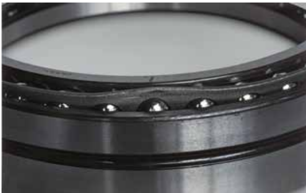
Photo 6.7.5 Part: Cage of an angular contact ball bearing Symptom: Pressed-steel cage deformation Cause: Shock load due to poor handling
