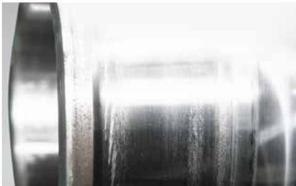
Photo 6.5.5 Part: Inner ring of a spherical roller bearing Symptom: Partial smearing occurs circumferentially on raceway surface Cause: Poor lubrication
