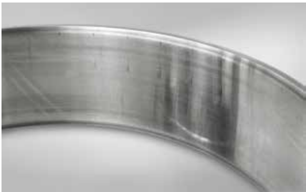
Photo 6.17.2 Part: Outer ring of a double-row cylindrical roller bearing Symptom: Axial scratches at roller pitch intervals on raceway surface Cause: Inclination of inner and outer rings during mounting
