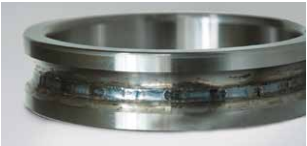
Photo 6.14.3 Part: Inner ring of an angular contact ball bearing Symptom: Raceway discoloration, melting occurs at ball pitch intervals Cause: Excessive preload
