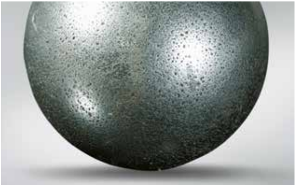
Photo 6.9.2 Part: Ball of Photo 6.9.1 Symptom: Pitting occurs on the rolling element surface
