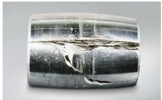
Photo 6.6.8 Part: Roller of a spherical roller bearing Symptom: Axial cracks occur on rolling surface
