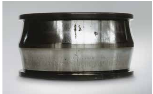
Photo 6.6.6 Part: Inner ring of a spherical roller bearing Symptom: Axial cracks occur on raceway surface Cause: Large fitting stress due to temperature difference between shaft and inner ring
