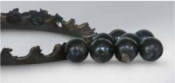
Photo 6.14.5 Part: Balls and cage of Photo 6.14.3 Symptom: Cage is damaged by melting, balls become discolored and melted Cause: Excessive preload
