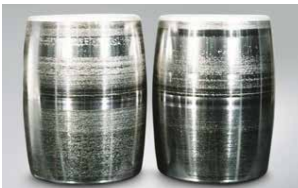
Photo 6.5.7 Part: Convex rollers of Photo 6.5.5 Symptom: Smearing occurs at the center of the rolling surface Cause: Poor lubrication
