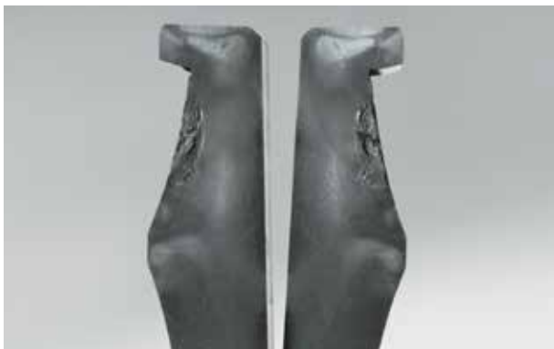
Photo 6.6.7 Part: Cross section of a fractured inner ring in Photo 6.6.6 Symptom: Origin is directly beneath the raceway surface
