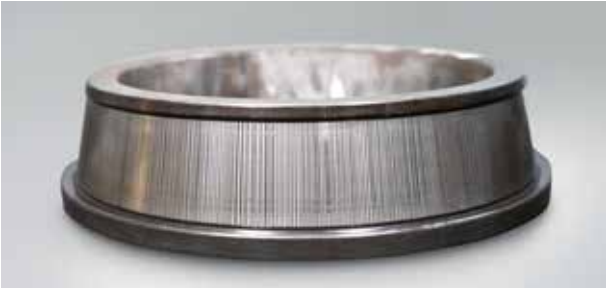
Photo 6.15.1 Part: Inner ring of a tapered roller bearing Symptom: Striped pattern of corrosion occurs on the raceway surface
