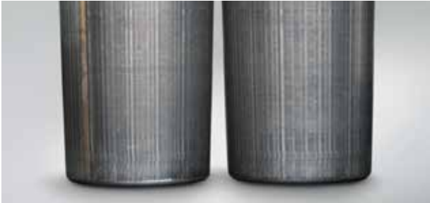
Photo 6.15.2 Part: Tapered rollers in Photo 6.15.1 Symptom: Striped pattern of corrosion occurs on the rolling surface
