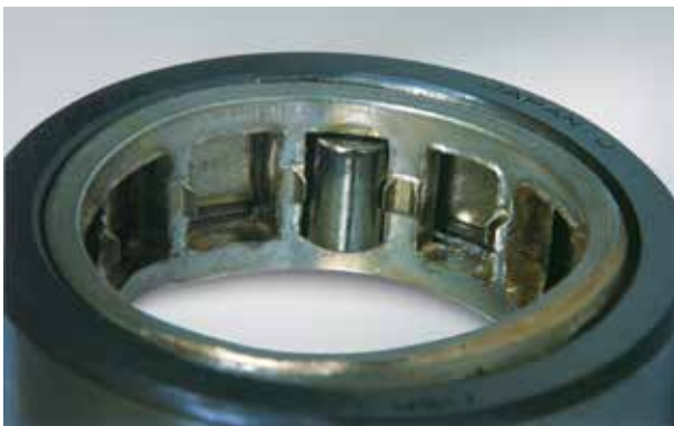
Photo 6.7.7 Part: Cage of a cylindrical roller bearing Symptom: Deformation and wear of a machined high-tension brass cage
