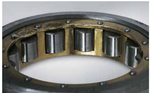
Photo 6.7.6 Part: Cage of a cylindrical roller bearing Symptom: Deformation of the side face of a machined high-tension brass cage Cause: Large shock during mounting
