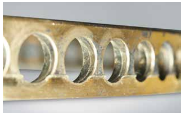
Photo 6.7.8 Part: Cage of an angular contact ball bearing Symptom: Stepped wear on the outside surface and pocket surface of a machined high-tension brass cage
