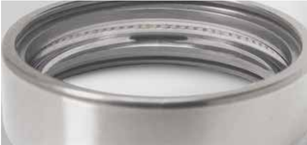
Photo 6.15.6 Part: Outer ring of a deep groove ball bearing Symptom: Fluting occurs on the raceway surface (high frequency)
