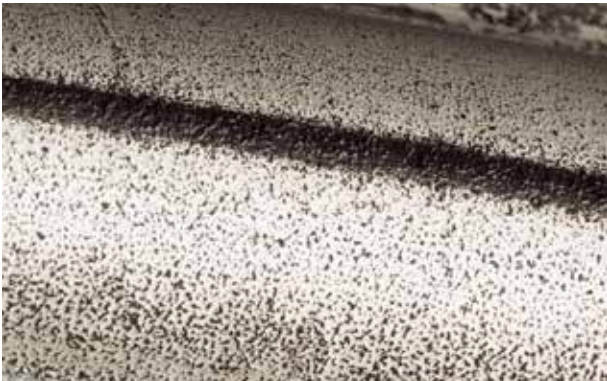
Photo 6.9.1 Part: Outer ring of a slewing bearing Symptom: Pitting occurs on the raceway surface Cause: Rust at bottoms of indentations
