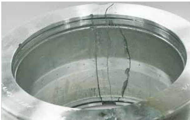
Photo 6.6.5 Part: Raceway surface of outer ring in Photo 6.6.4 Symptom: Outside surface crack developing on the raceway
