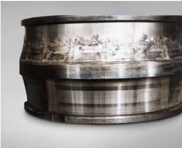
Photo 6.14.1 Part: Inner ring of a spherical roller bearing Symptom: Raceway is discolored and melted. Worn particles from the cage were rolled and attached to the raceway Cause: Insufficient lubrication
