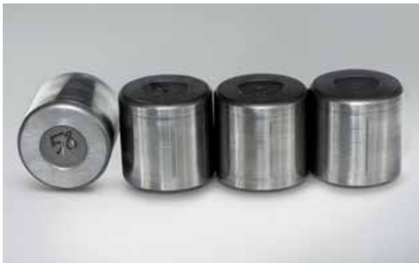
Photo 6.17.3 Part: Rollers of a cylindrical roller bearing Symptom: Axial scratches on rolling surface Cause: Inclination of inner and outer rings during mounting
