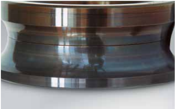
Photo 6.18.2 Part: Inner ring of a 4-point contact ball bearing Symptom: Bluish or purplish discoloration on raceway surface Cause: Heat generation due to poor lubrication
