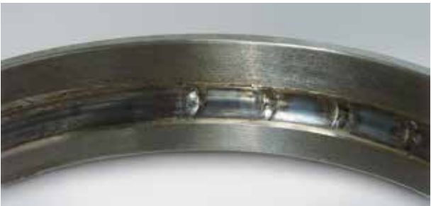
Photo 6.14.4 Part: Outer ring in Photo 6.14.3 Symptom: Raceway discoloration, melting occurs at ball pitch intervals Cause: Excessive preload
