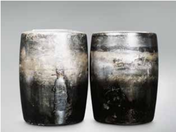
Photo 6.14.2 Part: Convex rollers of Photo 6.14.1 Symptom: Discoloration and melting of roller rolling surface, adhesion of worn particles from cage Cause: Insufficient lubrication
