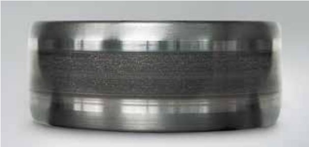
Photo 6.15.3 Part: Inner ring of a cylindrical roller bearing Symptom: Belt pattern of electrical corrosion accompanied by pits on the raceway surface
