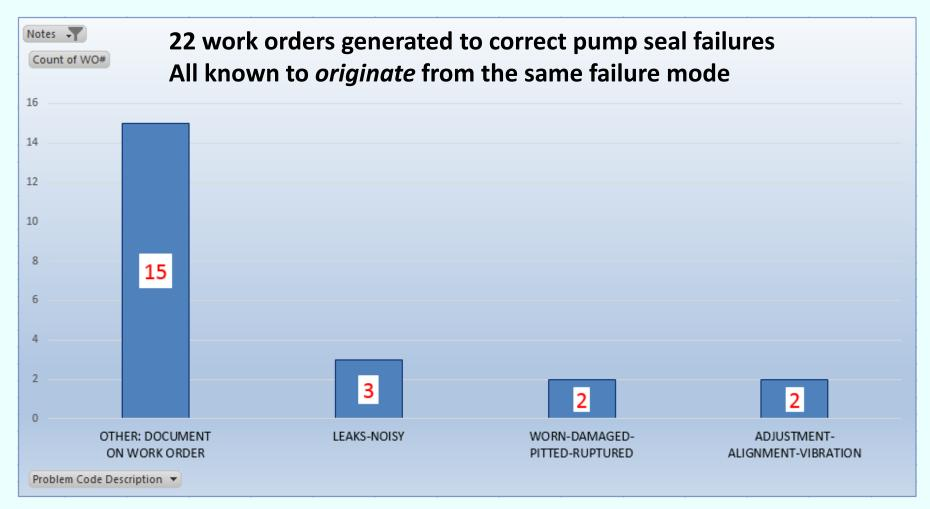
Inconsistently applied codes makes failure trending extremely difficult
